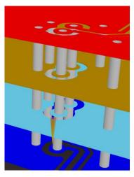
From the picture you can see that when a via is not set up properly, there can be pads around the via on inner layers. These pads cause a non-uniform E-field between the via tube and both the ground vias/pour as well as the other signal via.
