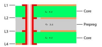
Because of the different dielectric constants of the materials in the stackup shown, there would be different capacitances between the via and any reference plane. E. g. C12 would not be the same as C23.
