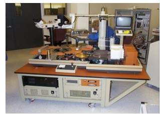
8 inch wafer probe station. The system is used to load and manipulate wafers. Most of this activity is performed under a microscope. Bond pads and tungsten tips are extremely difficult to see with the naked eye.
