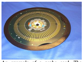
An example of a probe card. The strips of gold are contact points to the ATE. The center of the card contains the probe tips which make contact to the bond pads of the wafer.
