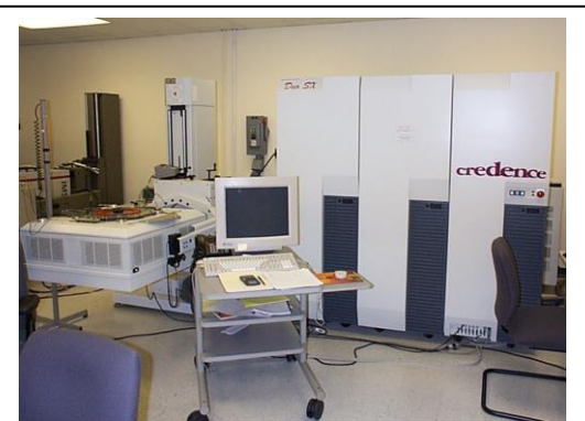
This is the Credence ATE Duo System. It is capable of testing a device with 512 I/Os. The unit is composed of a SPARC station, test head (on the far left) and a bay which houses the logic boards of the systems.
