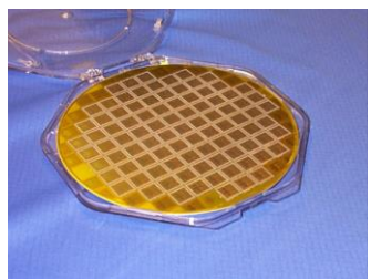
An example of an 8 in. wafer. Each square is an individual die. Through the use of a probe card, prober and ATE, each die can be tested without having to cut the wafer.
