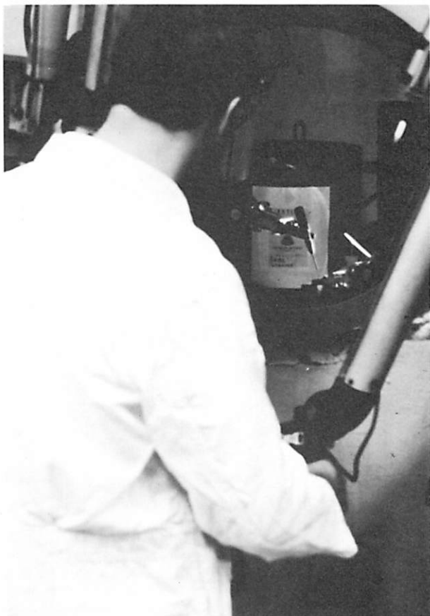
Reprocessing technician operates mechanical arms
