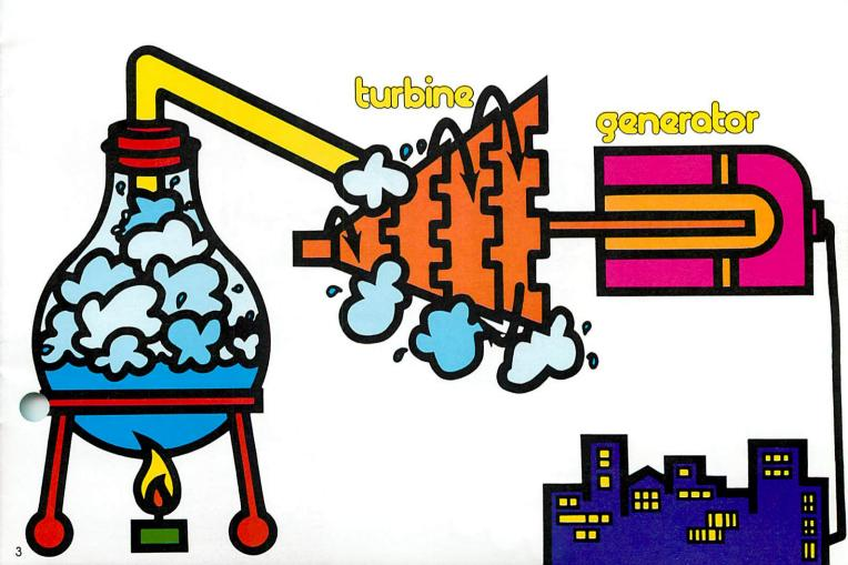
A fossil fuel power plant makes electricity using this principle. A fossil fuel plant burns coal, oil, or gas to heat water. As the fossil fuel is burned, the heat produced changes the water in the boiler to steam, and this steam is used to turn a turbine. In this manner, heat energy is converted into rotational energy. The turbine then turns a generator which makes electricity.
