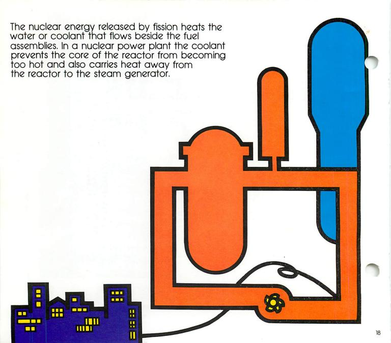
In a pressurized water reactor, the system of piping which contains the coolant is called the primary side. The separate system of piping where steam is produced to spin the turbine is called the secondary side. The primary system water and the secondary system water do not mix. Instead, the heated primary system water flows through the tubes of the steam generator which are surrounded by the cooler secondary system water.
