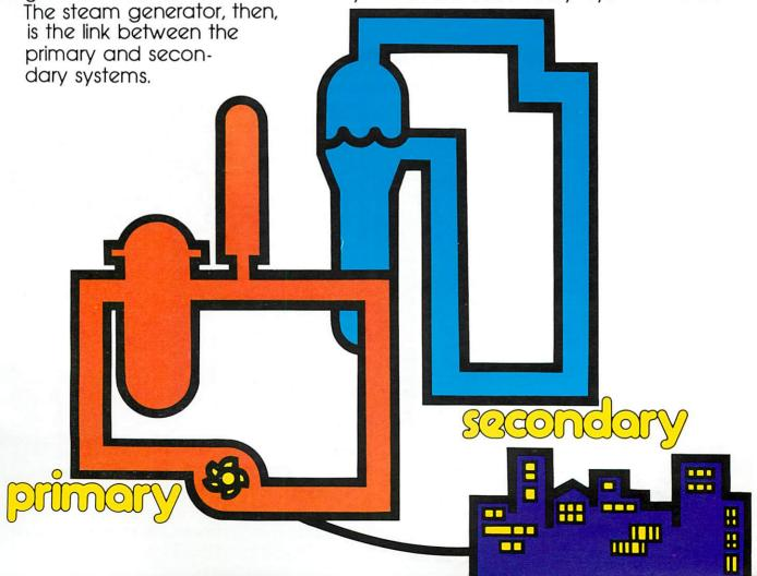
In a nuclear power plant, a vessel known as a pressurizer keeps the primary side at high pressure to prevent boiling yet allow water temperatures to reach 600°F. Since the primary system water is much hotter than the secondary system water, it easily boils the secondary system water to steam which turns the turbine.
