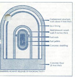
reactor could lose coolant water, leaving the super-hot reactor core at least partially uncovered. This would cause heat to build up within minutes. The zirconium rods would then be corroded away, leaving the fuel exposed. When the temperature reached 5000 degrees Fahrenheit, the fuel would turn molten, and a white-hot viscous mass would form inside the pressure vessel.
