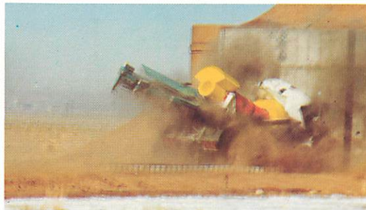
LATER, THE SAME CASK was slammed into the concrete wall at 84 mph.
