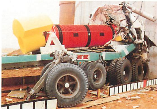
WHILE THE TRUCKS were totally demolished, the container suffered only a few dents.
