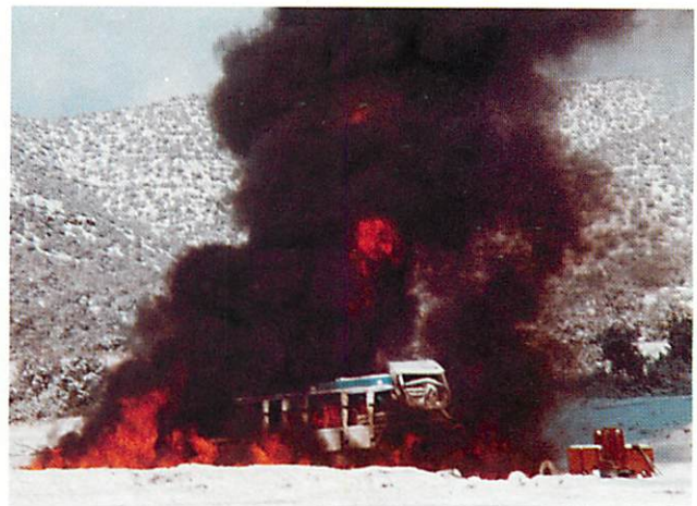
IN ONE OF its latest tests, Sandia engulfed a 74-ton shipping cask in burning jet fuel for a half-hour at temperatures between 1800 and 2100°F. The casks did not leak.
