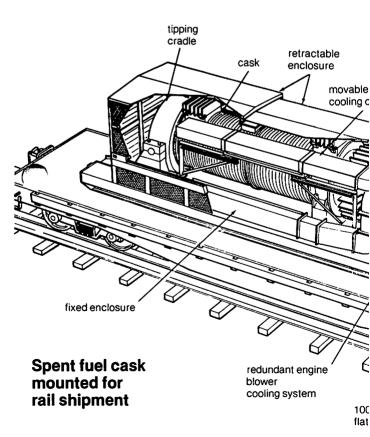
Due to these and other safety features, more than 5,000 spent nuclear fuel assemblies have been shipped without a single injury due to a release of radioactivity.
