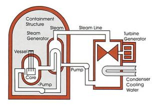
In a light water reactor, the type of nuclear power plant built in the United States today, the heat is taken away by continuously circulating water. The water moves through the reactor vessel, takes heat from the fuel rods, and then proceeds to a steam generator, where it gives up its heat. Cooler now, the water returns to the reactor vessel to do its job again . . . and again and again. The steam produced in the steam generator turns the turbine to make electricity.
