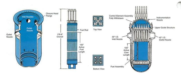
Units 2 and 3 contain about 112 tons of slightly enriched uranium dioxide. The uranium dioxide pellets, about one-third of an inch in diameter, are contained in fuel rods (tubes) about 12 feet long. The fuel rods, in turn, are assembled into clusters known as "fuel assemblies." One fuel loading of 217 "fuel assemblies" is equivalent in heat output to approximately 43 million barrels of fuel oil or 243 billion cubic feet of natural gas.
